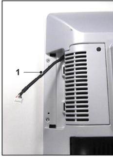
1. Remove the flap using a screw driver, exposing one end of a connecting cable (1).
