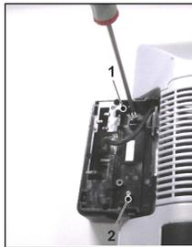
5. Use the two screws supplied to secure the holder to the display, in locations (1) and (2).
