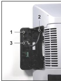
4. Locate the holder (1) to the side of the display uncovered in step 1.
